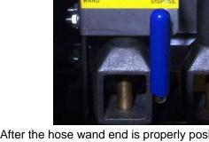
After the hose wand end is properly positioned in the frypot, activate the filter pump by turning the blue handle to "WAND" (where applicable).
